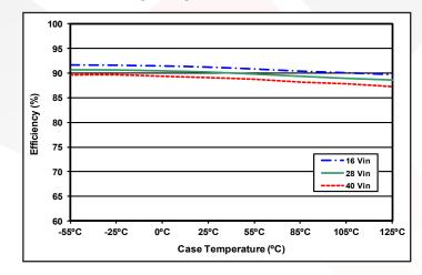
Figure 5: Efficiency at 60% load (7.2 A load on +5V and 7.2 A load on -5V) versus case temperature for Vin = 16V, 28V, and 40V.
