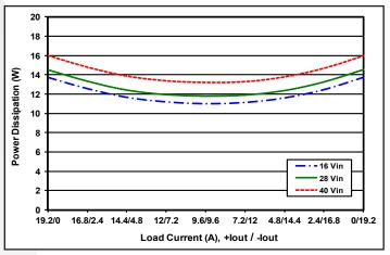
Figure 4: Power dissipations vs. output current, with total output current fixed at 80% load (96 W) and loads split as shown between the +5V and -5V outputs at minimum, nominal, and max input voltage at 25°C.
