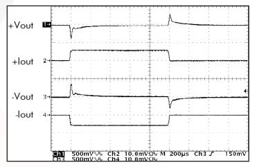
Figure 18: Output voltage response to step-change in total load current (0%-50%-0%) of total lout (max) split 50% / 50%. Load cap:  $1\mu$ F ceramic cap and  $10\mu$ F, 100 m $\Omega$  ESR tantalum cap. Ch 1: +Vout (500mV/div); Ch 2: +Iout (10AV/div); Ch 3: -Vout (500mV/div); Ch 4: -Iout (10A/div).
