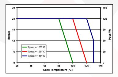
Figure 11: Output Current / Output Power derating curves as a function of Tcase and the maximum desired power MOSFET junction temperature at Vin = 28V (see Note 15).
