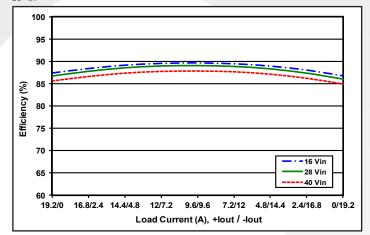
Figure 3: Efficiency vs. output current, with total output current fixed at 80% load (96 W) and loads split as shown between the +5V and -5V outputs at minimum, nomina, and maximum input voltage at  $25^{\circ}$ C.
