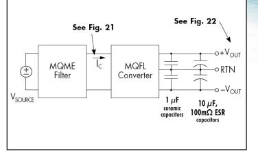
Figure 20: Test set-up diagram showing measurement points for Input Terminal Ripple Current (Figure 21) and Output Voltage Ripple (Figure 22).
