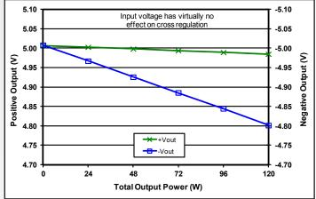
*Figure 10: Load regulation vs. total output power from zero to full load where -lout equals three times +lout at nominal input voltage and Tcase 25°C.*
