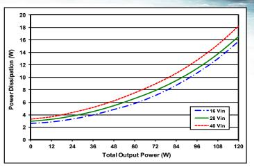
Figure 2: Power dissipation vs. output power, from zero to full load with equal load on the +5V and -5V outputs at minimum, nominal, and maximum input voltage at  $25^{\circ}$ C.
