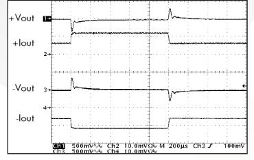
Figure 17: Output voltage response to step-change in total load current (50%-100%-50%) of total lout (max) split 50% / 50%. Load cap:  $1\mu$ F ceranic cap and  $10\mu$ F, 100 m $\Omega$  ESR tantalum cap. Ch 1: +Vout (500mV/div); Ch 2: +Iout (10AV/div); Ch 3: -Vout (500mV/div); Ch 4: -Iout (10A/div).
