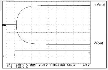
Figure 15: Turn-on transient at full rated load current (resistive laod) (5 ms/ div). Input voltage pre-applied. Ch 1: +Vout (2V/div); Ch 2: -Vout (2V/div); Ch 3: Enable2 input (5V/div).
