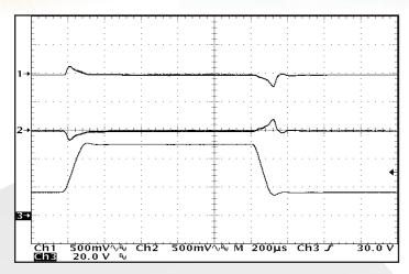
Figure 19: Output voltage response to step-change in input voltage (16V-50V-16V). Load camp:  $10\mu$ F, 100 m $\Omega$  ESR tantalum cap and  $1\mu$ F ceramic cap. Ch 1: +Vout (500mV/div); Ch 2: -Vout (500mV/dis); Ch 3: Vin (20V/div).
